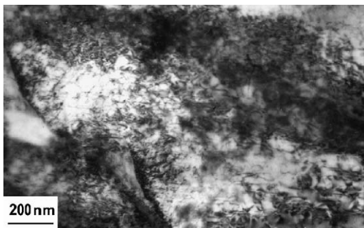
Fig. 4. Microstructure of steel 18Cr10NiTi irradiated by helium ions with energy 12 \text{ keV} at room temperature up to the dose 1 \times 10^{16} \text{ cm}^{-2} .
