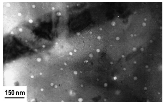
Fig. 6. Microstructure of steel 18Cr10NiTi irradiated by helium ions with energy 12 \text{ keV} at room temperature to a dose 2 \times 10^{15} \text{ cm}^{-2} and annealed at 1170 \text{ K} for 1800 \text{ s} .
